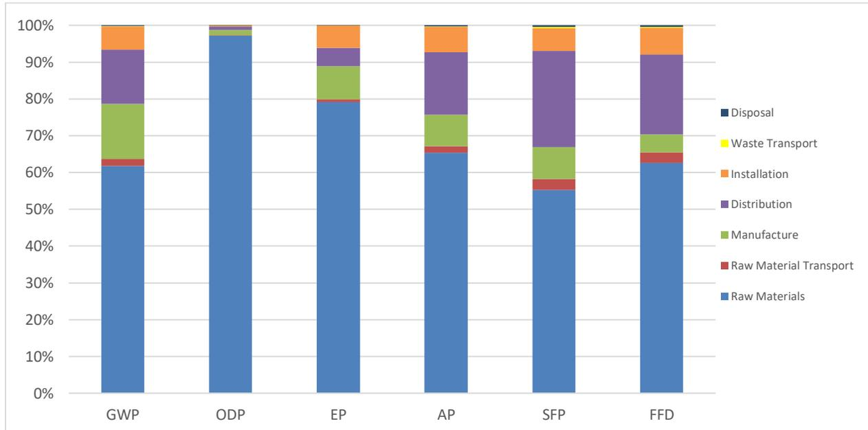
Figure 4. Contribution analysis without Use phase for P3TEC Advanced Wall Protection (TRACI).
