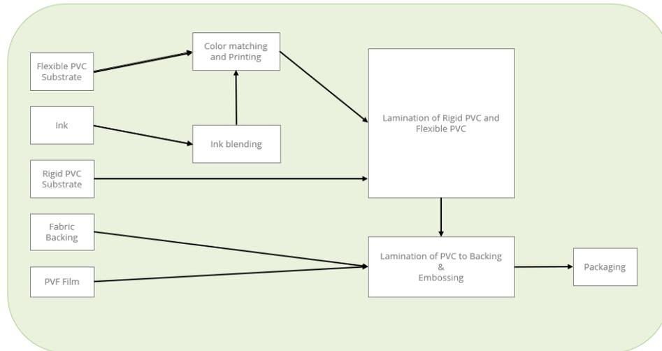
Figure 1. Manufacturing diagram for P3TEC Advanced Wall Protection.
